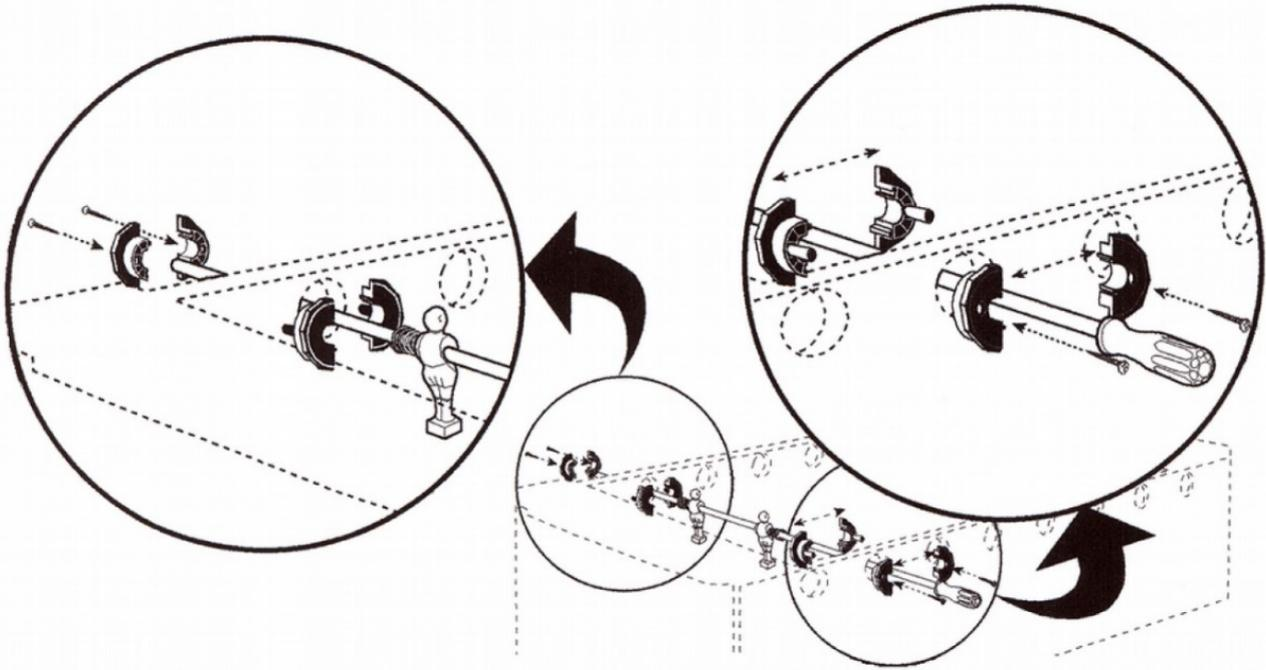
6. If not already fitted, attach the white & grey score cubes to the top of the ends of the table with the 4 long screws provided.
