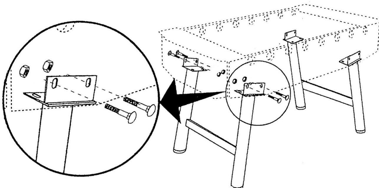
Insert the coach bolts into the sides of the table followed by a nut. The square neck of the bolt will not fit into the round hole. Tighten the nut so that the neck breaks into the laminate but do not over-tighten – this will not cause the laminate to crack. The mushroom head of the bolt should just touch the laminate surface.
